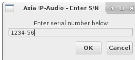
Enter the product serial number and then press the OK button. To obtain a serial number, contact Paravel Systems at [sales@paravelsystems.com](mailto:sales@paravelsystems.com), following which the configuration screen will appear. (Depending upon the specific product purchased, the appearance of the configuration dialog may vary from what is pictured here).
