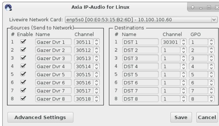
Select the network interface that is connected to the Livewire network from the Livewire Network Card dropdown list.
